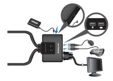
Connect your powered speaker and mic. to the console audio port and console mic. port.
